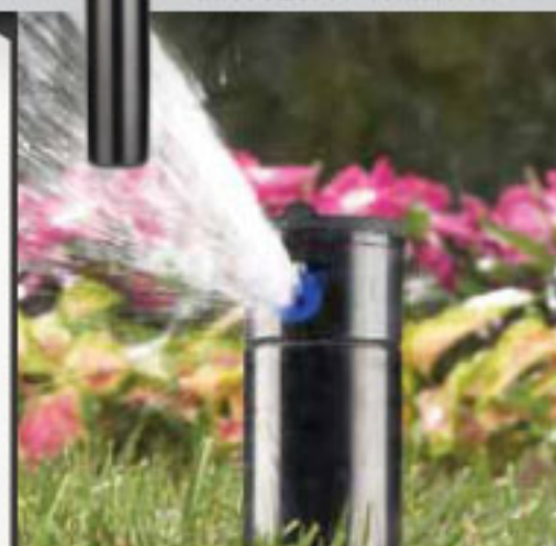
PGP-12: Overall height: 17" Pop-up height: 12" Exposed diameter: 1¾" Inlet size: ¾" female NPT
